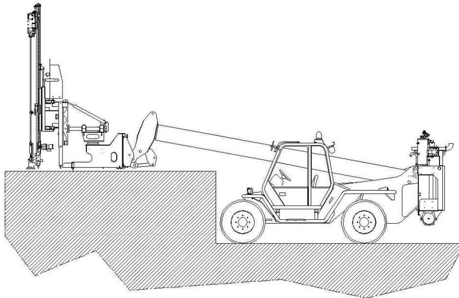
*Handy Maxidrill* is a hydraulic drilling mobile unit, totally independent, and suitable for vertical drilling on any inclined and in any type of rock.
